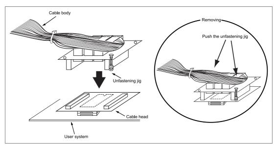
Figure 4 Fastening Cable Body
